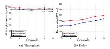
Fig. 17. Performance of the  $A^*$  algorithm when the channel has a BER of  $10^{-5}$ . Physical layer data and basic rates are 54 and 6 Mbps. Here the AP throughput percentage is the ratio between the throughput achieved using the  $A^*$  algorithm and the maximum throughput using fixed size buffers.
